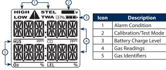
When a Gas Reading (4) exceeds its alarm threshold, the detector will go into visual, vibrating and audible alarm. On the display, the  $\triangle$  icon will appear beside the Alarm Condition (1) and the associated Gas Identifier (5) will flash off and on continuously.
